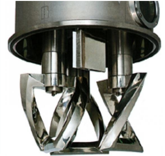
Dry powder blending and Solid / liquid mixing (High shear force)
