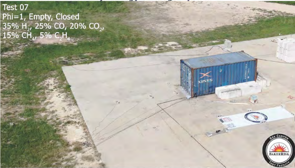
資料來源: Battery Energy Storage Systems - thermal runaway and explosion testing for Lithium-ion battery gas ( Video source )
